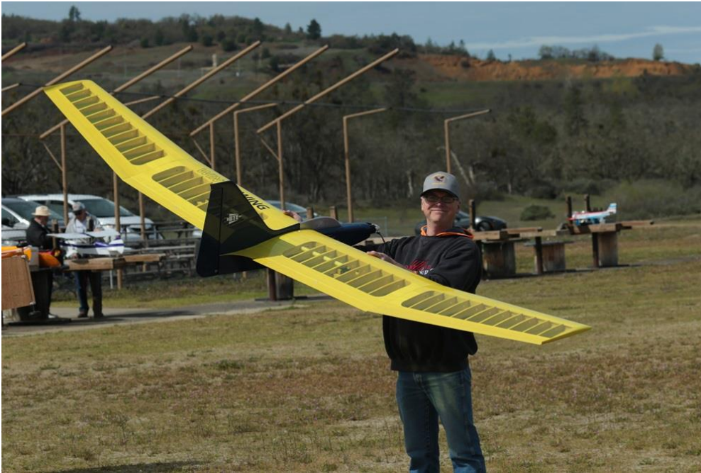
I designed, built, and flew this WinterWing for the 2019 Rogue Eagles Winter Build Challenge. The electric flying wing featured elevons and could be flown with or without the removable outer wing panels. Used dolly for takeoff. (Photo provided by Bruce A. Tharpe. Photo taken by Rick Lindsey.)
