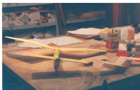
The latest scale home built model from Ron before he messed with the dihedral. A smaller dynamically similar glider is to the right of it; this was first made to find a good center of gravity location for the yellow Free Flight model. A large RC model is in the works.
