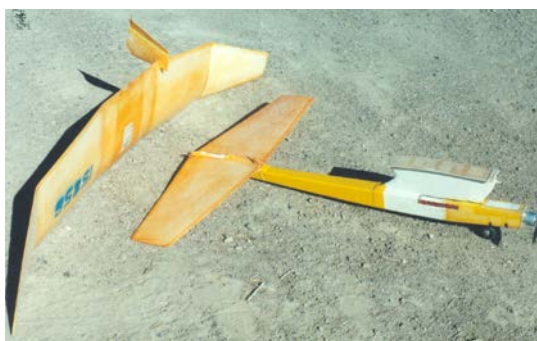
A larger SFC Odd-Rod showing a weird accident that actually happened – a normal landing in sage brush clean off the fin and somehow buried it in the wing's trailing edge!
