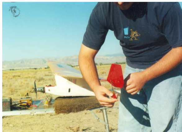
The test ship for wing fins (detachable) that demonstrated lack of performance improvement. The Radio Control (RC) model was first flown with no wing fins then the rudder was trimmed to result in a straight glide. One fin was installed after that to see if a turn would be induced because of increased lift and/or reduced drag. The result was that it still glided straight at the same trim setting on Tx – another great idea shot down!
