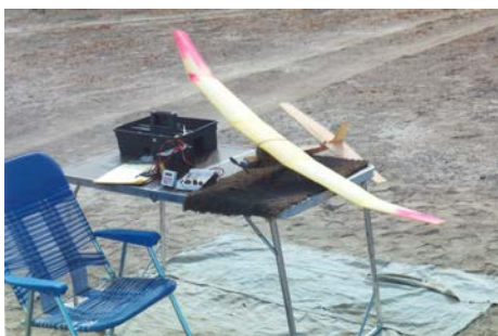
Another Ramrod derivative – this one with a swept-back wing 30% longer than original to increase the area and aspect ratio, which is a great way to go for an electric.
