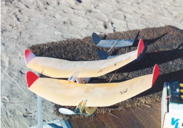
These two nearly identical micro-models were flight-compared to measure the differences between direct-drive and geared motors. What he found was that the geared job climbed slower, but the motor ran longer on the same battery charge (Cutie design).
