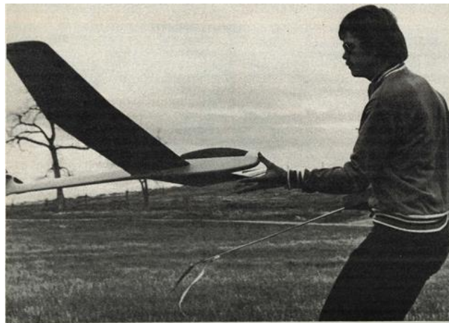
Nosing into its pilot's waiting hand, the Aquila flown by Miller had a wing modification, made two days before the Team Finals. The last-minute change was a daring gamble to make his ship move a bit faster than a stock Aquila and to beef up the structure for the rigorous speed runs
