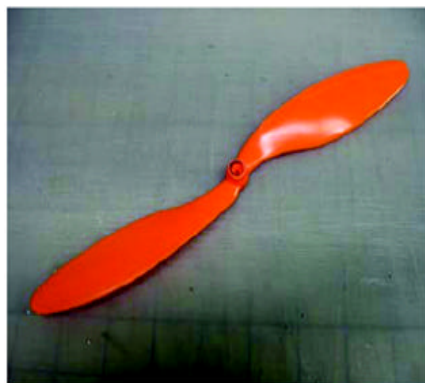
Stock 10-inch x 4.7-inch slow-fly propeller.
