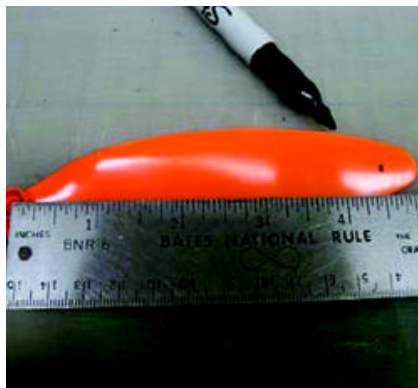
Measure 4.5 inches from the hub and mark.
