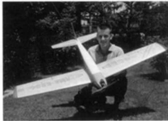
Top Flite Orion with K&B .45 engine and home built 8-channel reed R/C system + Bonner servos - 1960
