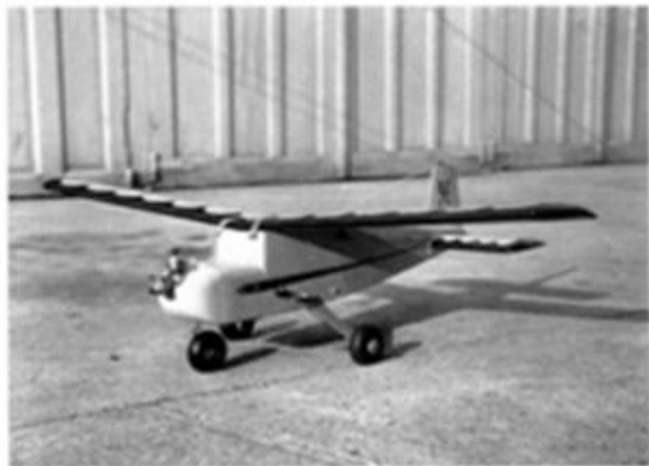
Original "Shookywukms" rudder only SN escapement R/C model with Webra .09 diesel engine - 1956
