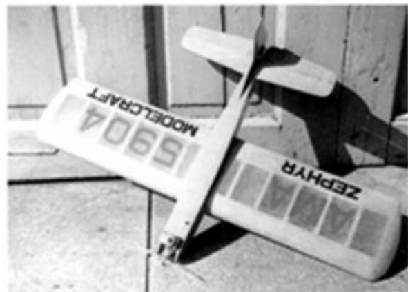
1/2A scratch-built CL stunt plane with Alyn Sky Fury .049 engine - 1954
