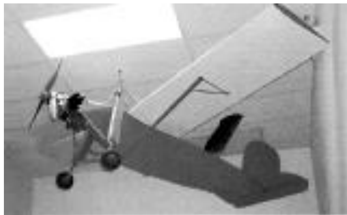
A restored OQ-2 drone before complete covering. Notice the stamped aluminum wing ribs and two propellers on one shaft contra-rotating via a gearbox.
